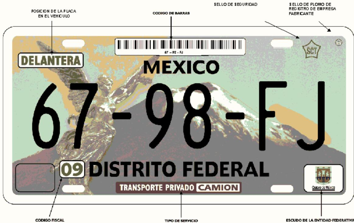
FIGURA 13 "MODELO DE PLACA CON 2 GUIONES Y 6 CARACTERES"
