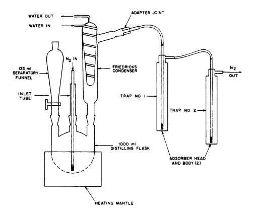
125 ml. separatory funnel with 24/40 joint (VWR Cat. No. 30357-102)Inlet tube with 24/40 joint (VWR Cat. No.
