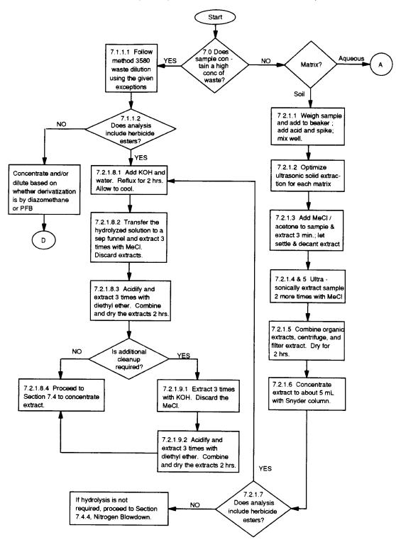
Extraction/Hydrolysis of Aqueous Samples and Extract Concentration
